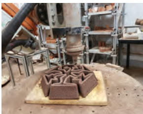
機械臂3D打印 Robot 3D printing
