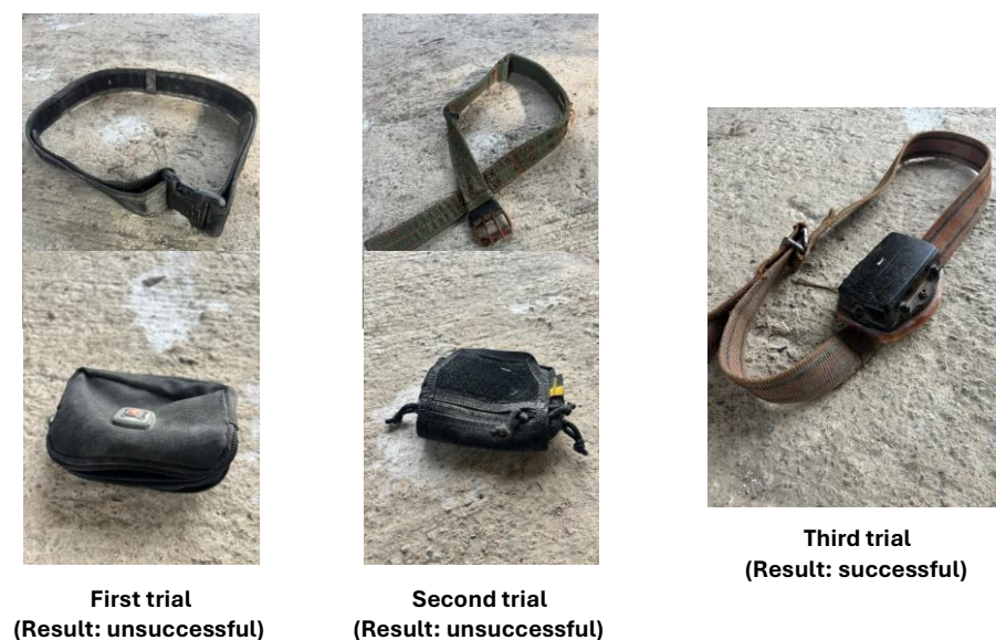
Figure 15. Trials of collar and tracker housing method
