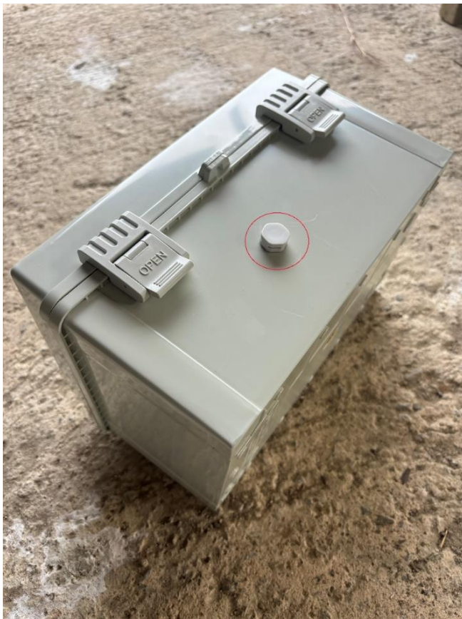
Figure 16. Waterproof box with exhaust hole
