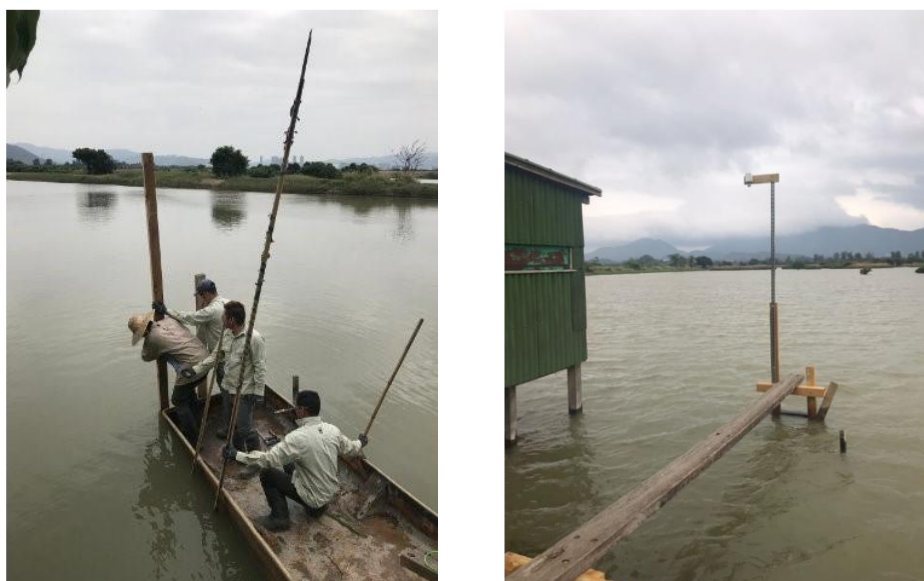
Figure 6. On-site deployment of water level sensor
