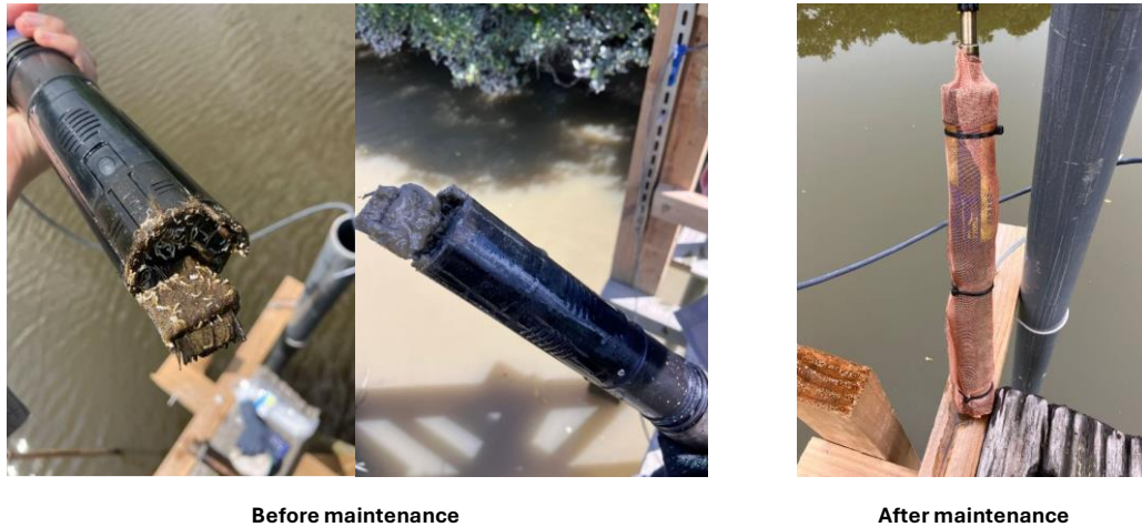
Figure 17. Water quality sensors before and after maintenance
