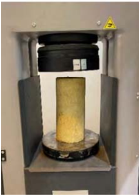
Compression test in HKUST
