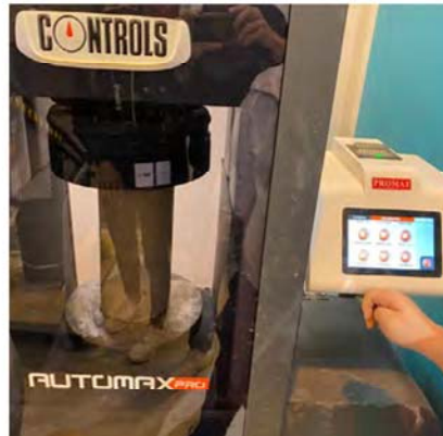
Preparing sample cylinder for compression test (The left sample was made with 1:1 soil-stone proportion while the right one has 1:2 soil-stone proportion.)
