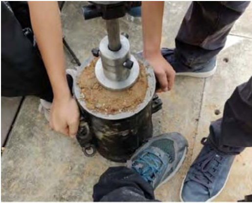
Preparing sample cylinder for compression test (The left sample was made with 1:1 soil-stone proportion while the right one has 1:2 soil-stone proportion.)
