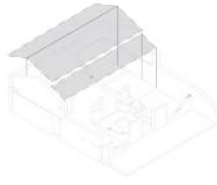
DOUBLE LAYER ROOF FOR VENTILATION AND NORTHLIGHT
