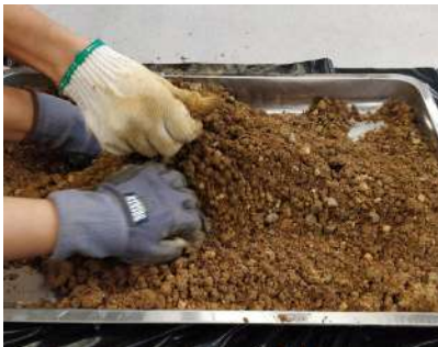
1. Mixing earth samples with water
