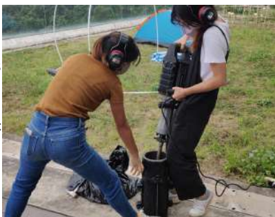
3. Compress the earth samples with electric hammer
