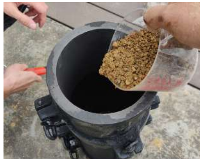
2. Pour wet earth samples into the metal cone-shaped mould
