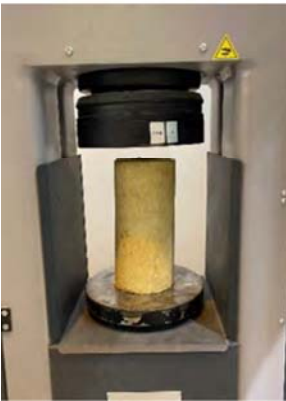
Compression test in HKUST
