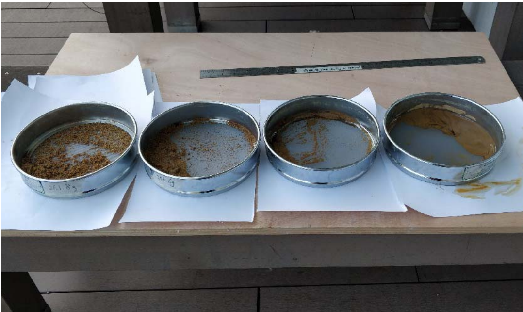
Dry sieving and wet sieving test by students
