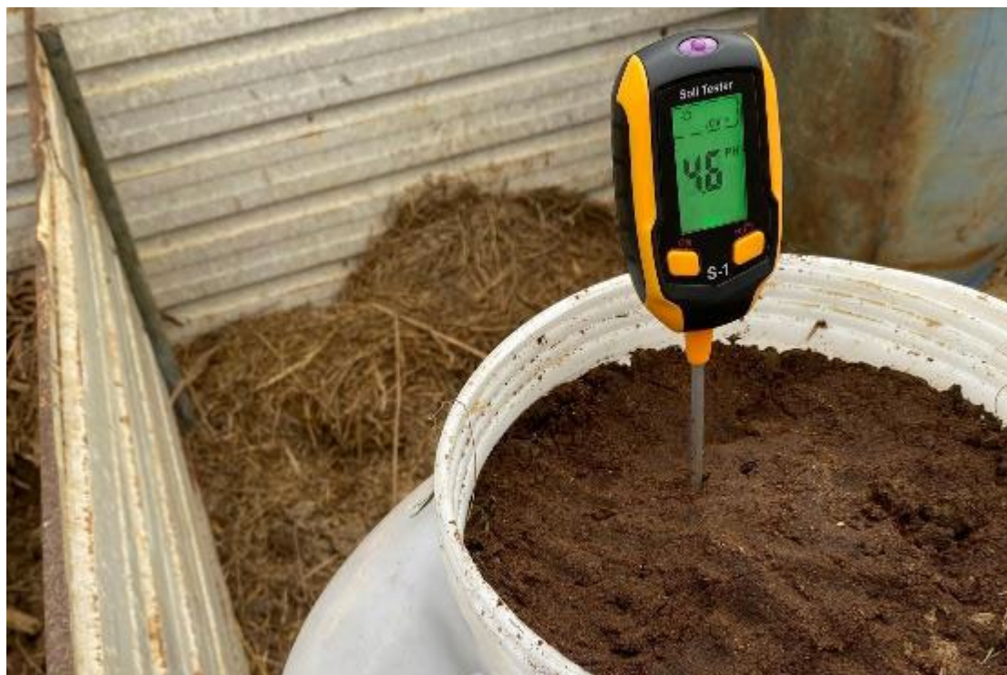
Photo 12. Measuring the pH value and temperature of the compost
